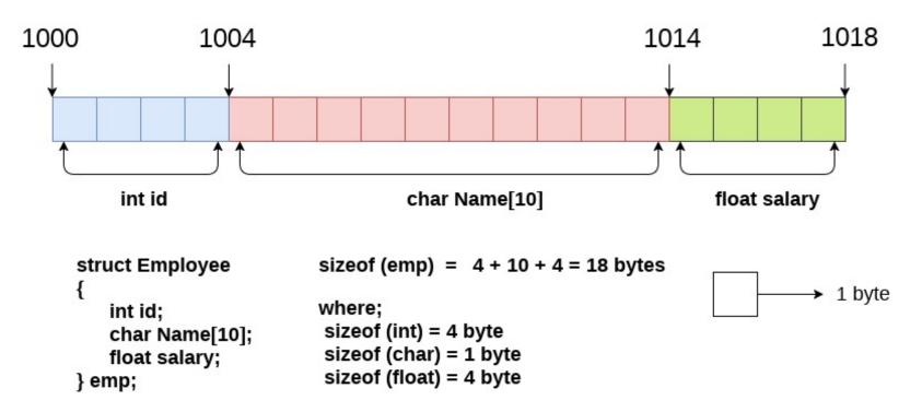
Here, **struct** is the keyword; **employee** is the name of the structure; **id**, **name**, and **salary** are the members or fields of the structure. Let's understand it by the diagram given below:
